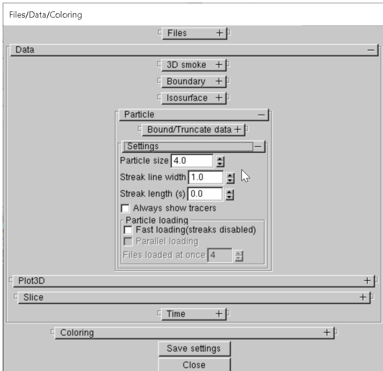
Figure 6.6: Dialog box for setting Particle file options. Select a variable and bound type. Enter a lower and/or upper bound if set bound type was selected. Particle files may be loaded in parallel by selecting the Fast loading checkbox and setting the number of files to load in parallel.
