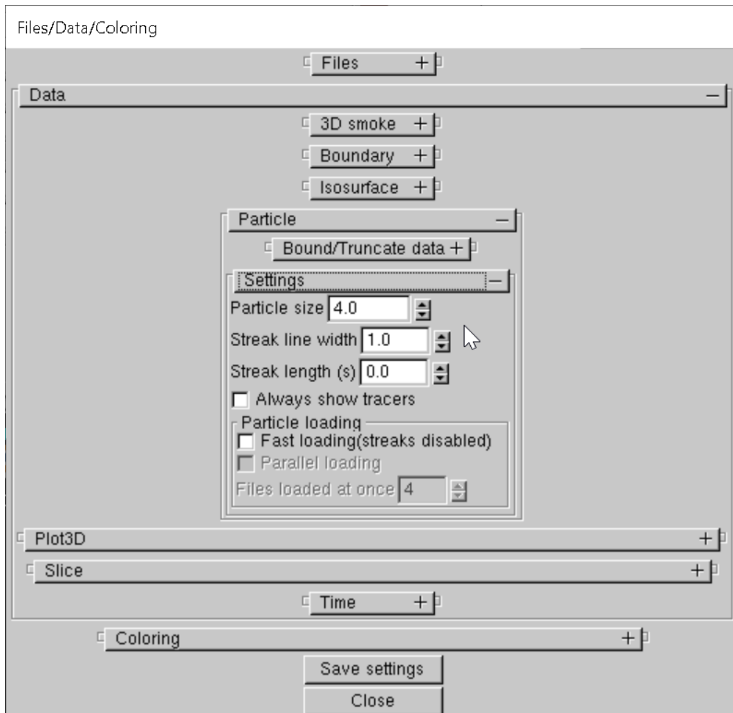
Figure 6.5: Dialog box for setting Particle file options. Select a variable and bound type. Enter a lower and/or upper bound if set bound type was selected. Particle files may be loaded in parallel by selecting the Fast loading checkbox and setting the number of files to load in parallel.
