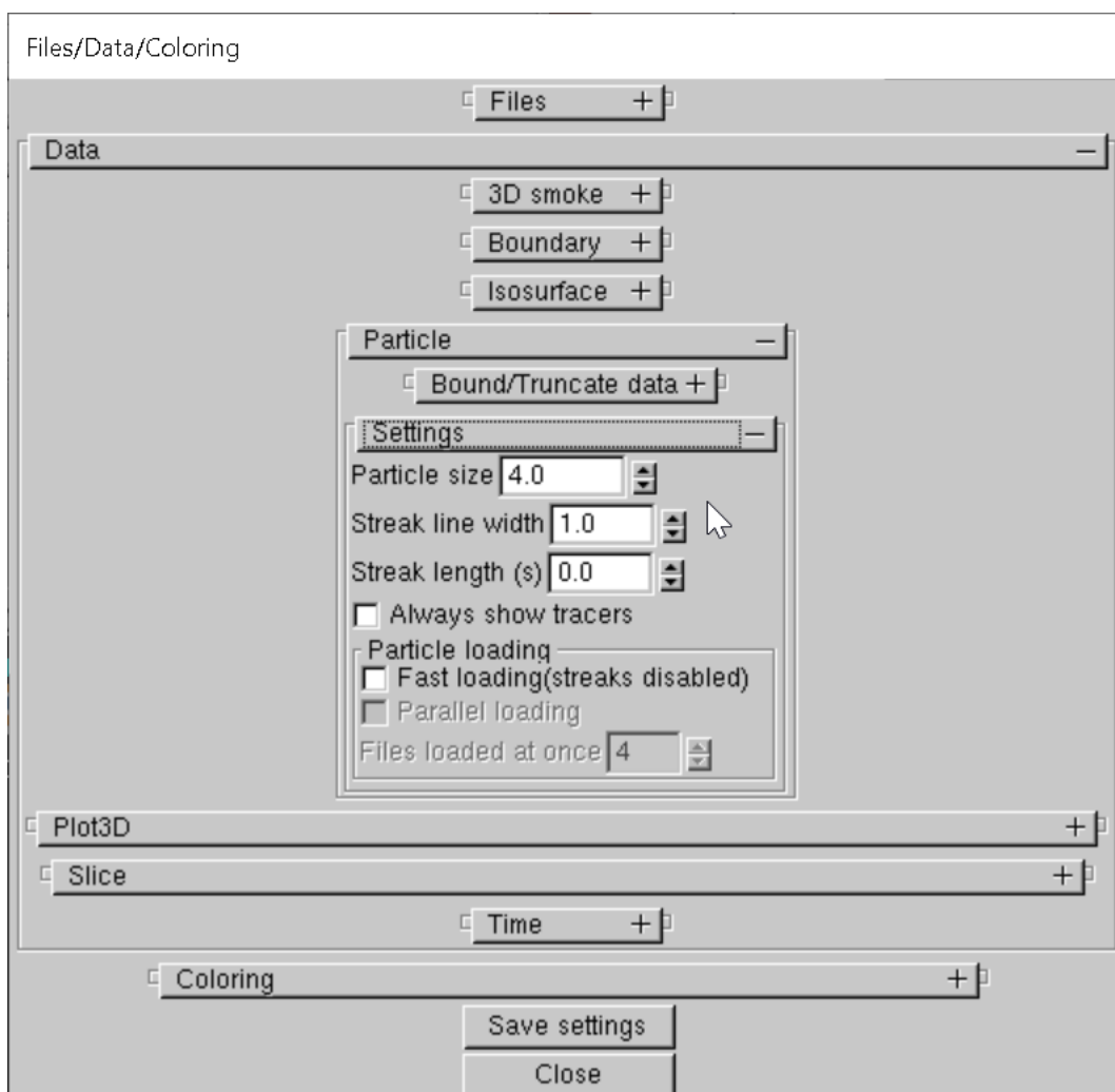
Figure 5.4: Dialog box for setting Particle file options. Select a variable and bound type. Enter a lower and/or upper bound if set bound type was selected. Particle files may be loaded in parallel by selecting the Fast loading checkbox and setting the number of files to load in parallel.
