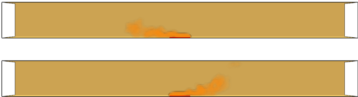
Figure 12.13: Snapshots from the sample case pressure_boundary showing a fire in a tunnel leaning left, then right, due to a positive, then negative, pressure imposed at the right portal.
