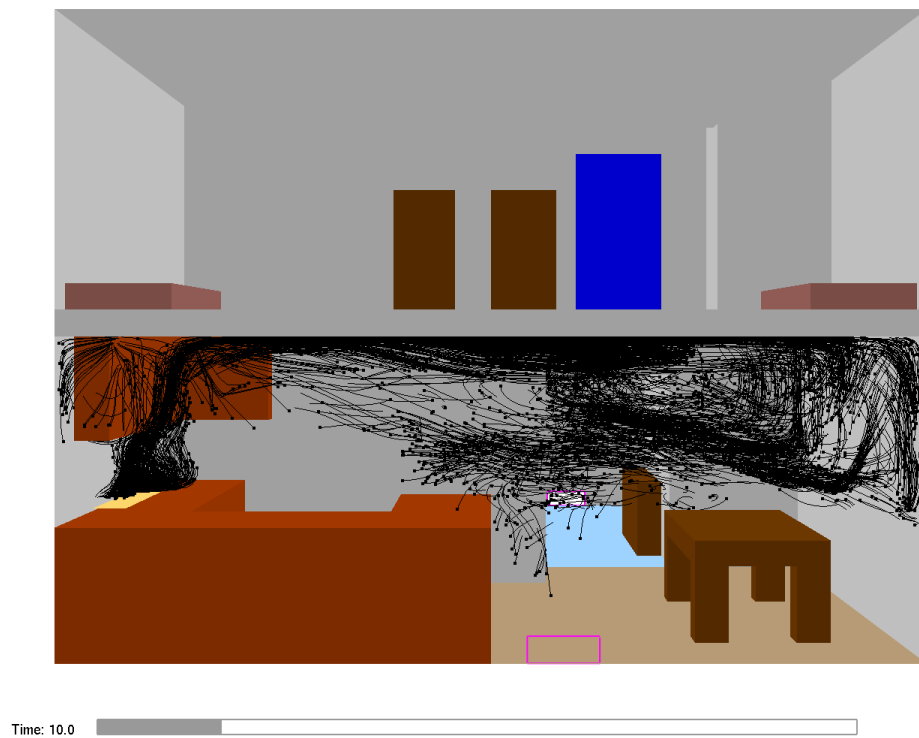
Figure 2.2: Townhouse kitchen fire visualized using streak lines. The pin heads shows flow conditions at 10 s, the corresponding tails shows conditions 1.0 s earlier.
