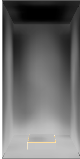
Figure 16.5: Wall soot deposition for the propane_flame_deposition test case.
